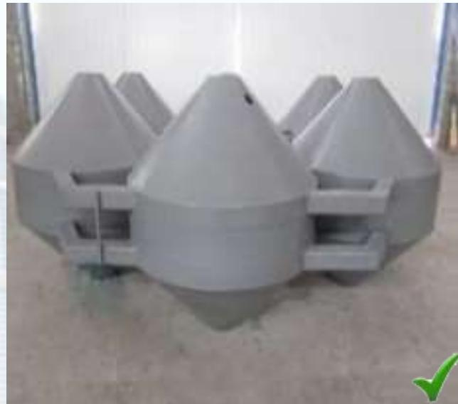
The innovative design of Super-Cell provides a very much lighter and easier to handle assembly which is readily secured inside the re-bar cage without the use of bearing plates, the cell-maker provides integral brackets or struts to give support for the cells inside the rebar cage.
