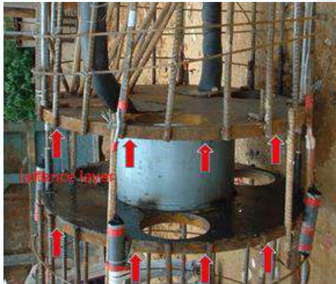
**.The hydraulic jack's cylinder and piston are welded to 50mm thick steel bearing plates. The bearing plate's flat surfaces become detrimental to the test function as they encourage build-up of a low strength laitance layer which affects the measured settlement. The Bearing plates can restrict the concrete flow inside the pile which can weaken the pile causing it to fail.**
