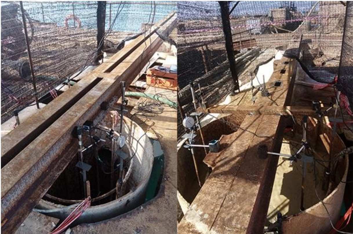
Test reference beam and instrumentation
